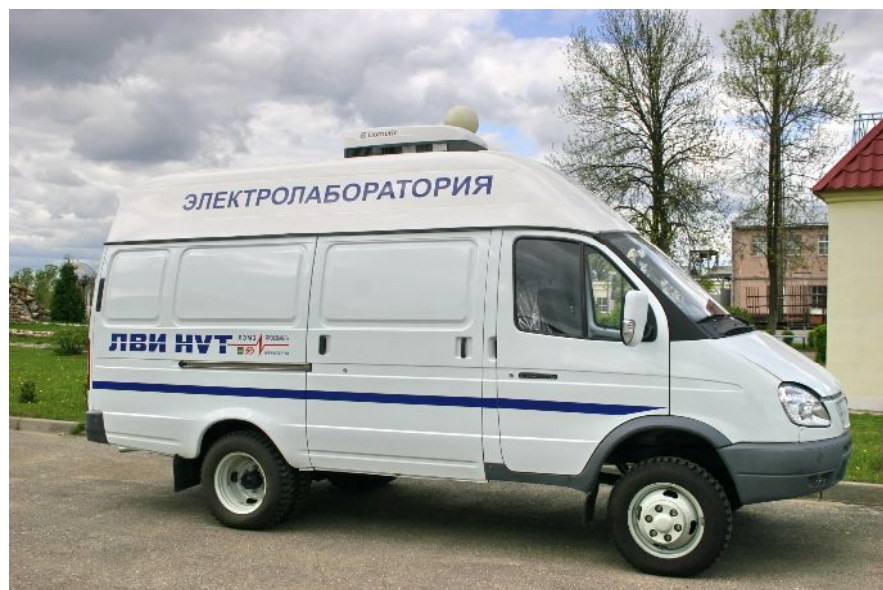
External view of the High Voltage Test Van LVI HVT -3FAVC on GAZ27057
