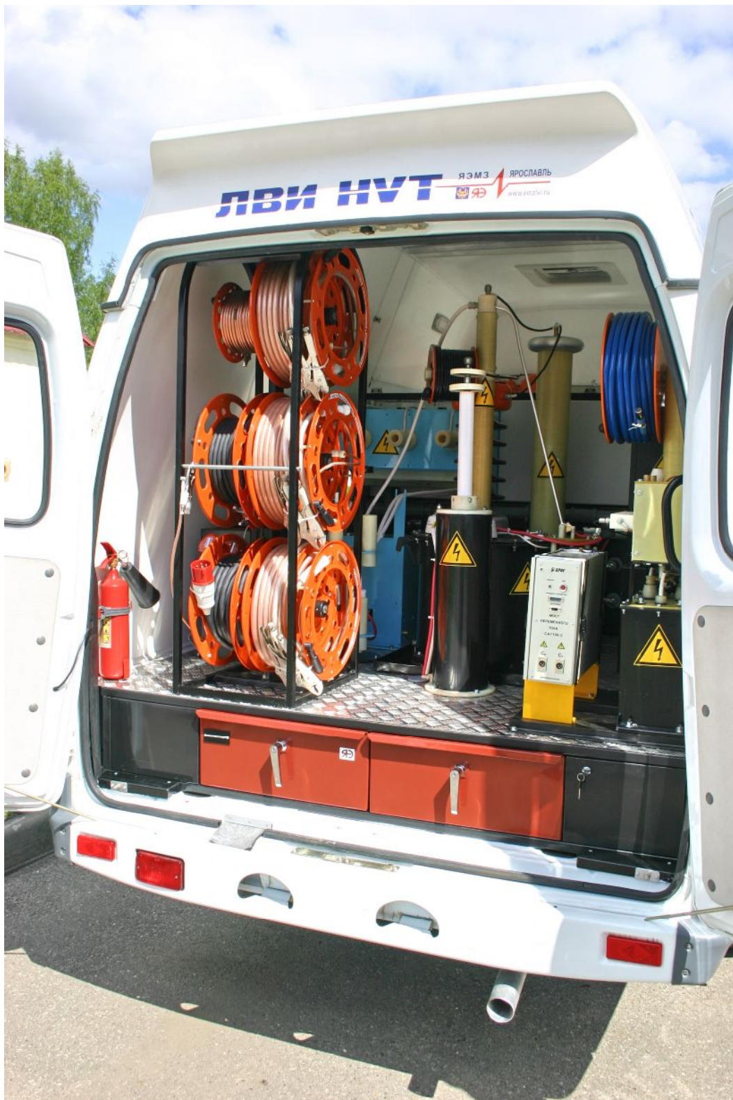
Views to the high voltage compartment of the laboratory LVI HVT-3FAVC on GAZ-27057
